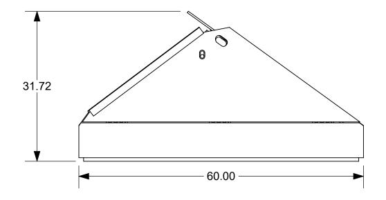
THIS FOLDABLE, MANUAL, WEDGE BARRIER IS DESIGNED TO BE EASILY MOBILE AND DEPLOYABLE ON EXISTING CONCRETE OR ASPHALT ROADWAYS OR SIDEWALKS. NO EXCAVATION OR SUB-SURFACE PREPARATION IS REQUIRED.
