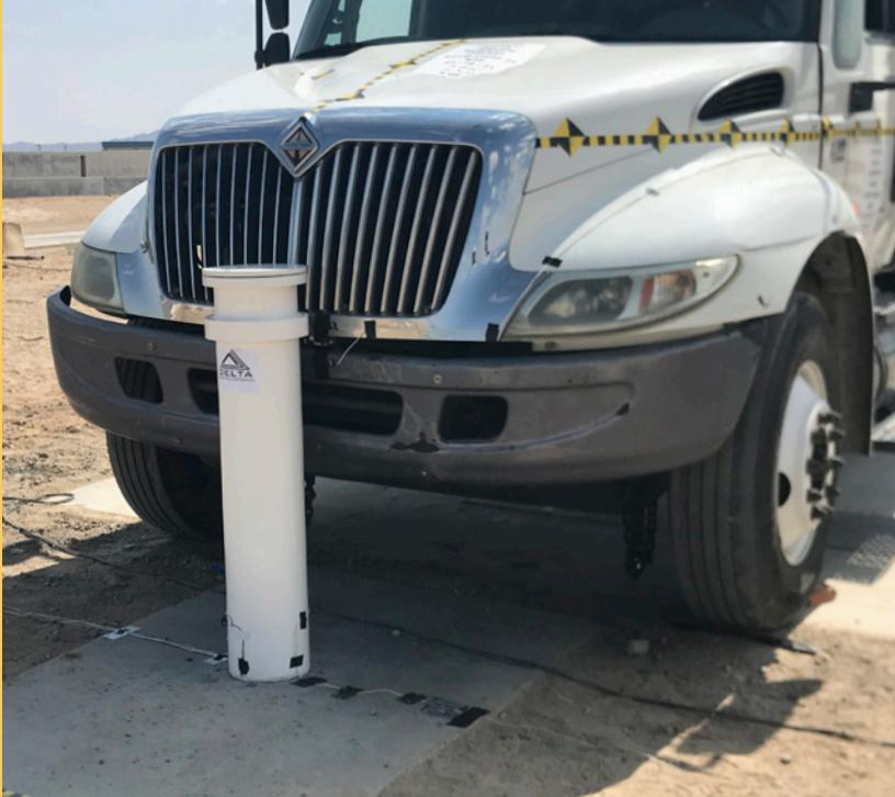
Delta Scientific's new DSC633 shallow foundation bollard has been successfully tested to ASTM F2656-20 M30/P1 standards. Designed for applications where underground utilities and space limitations pose a problem, the DSC633 is the perfect solution.
