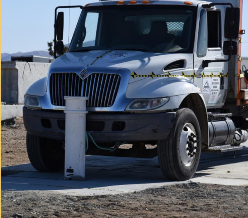
Delta Scientific's new DSC635 shallow foundation single bollard has been successfully tested to ASTM F2656-20 M50/P1 standards. Designed for applications where underground utilities and space limitations pose a problem, the DSC635 is the perfect solution.
