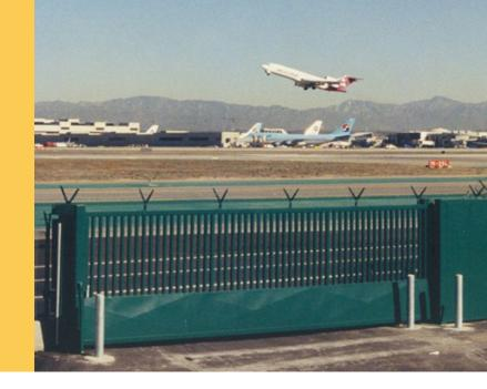
The cantilevered SC3000S sliding gate is ideal for locations that have ground interference and need the leaf of the gate suspended over the roadway. This rugged gate allows for railroad tracks or any other ground obstruction to easily pass underneath the gate leaf during opening and closing of the gate. The drive system can be either electric or hydraulic allowing for variable speeds and smooth operation.
