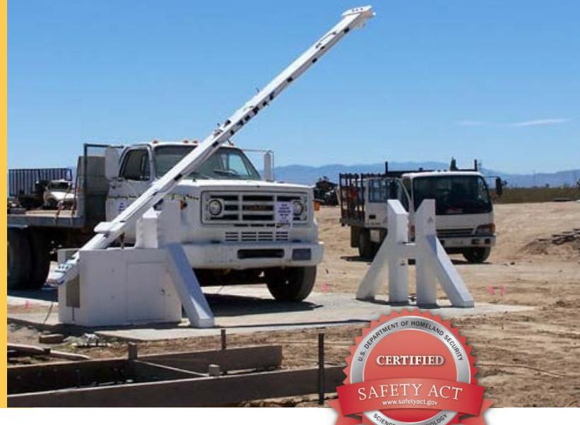
The DSC7000 crash rated beam barricade is used worldwide at locations where wide roadways need to be secured from attacking vehicles. It provides protection between 12- to 20-foot wide with options to 30 feet (3.7 to 9.2 m). The 725-pound beam of the vertical lift barricade stops a 15,000-pound (66.7 kN) vehicle traveling 50 mph (80 kph) dead in its tracks, equivalent to 1.2-million foot-pounds of kinetic energy.
