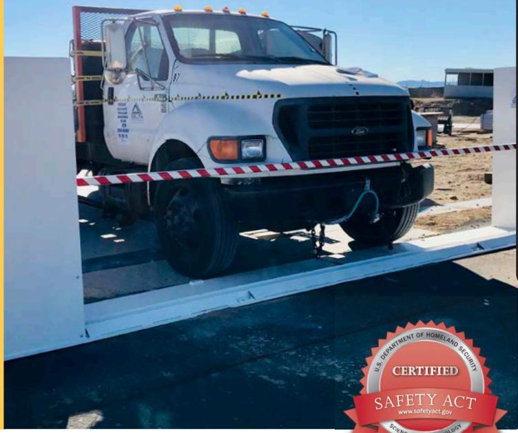
Delta's new DSC1500 portable beam barricade that sets up quickly and temporarily to block vehicles. The new portable barricade secures locations during short-term events and anywhere a beam barricade is needed for interim security. With a clear opening of 16 feet (4.8 m), the DSC1500 is M30 certified, able to stop a 15,000 pound (66.7 kN) vehicle going 30 mph (48 kph).
