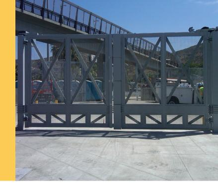
Delta Scientific's SGC1000 high security swing gate was designed to fill the need for a rugged manually operated crash-rated swing gate. The design of the end support assemblies add to its crash rated performance. A ground track is not needed. The SGC1000 provides a clear opening of 12 to 30 feet (3,657 mm to 9,144 mm).
