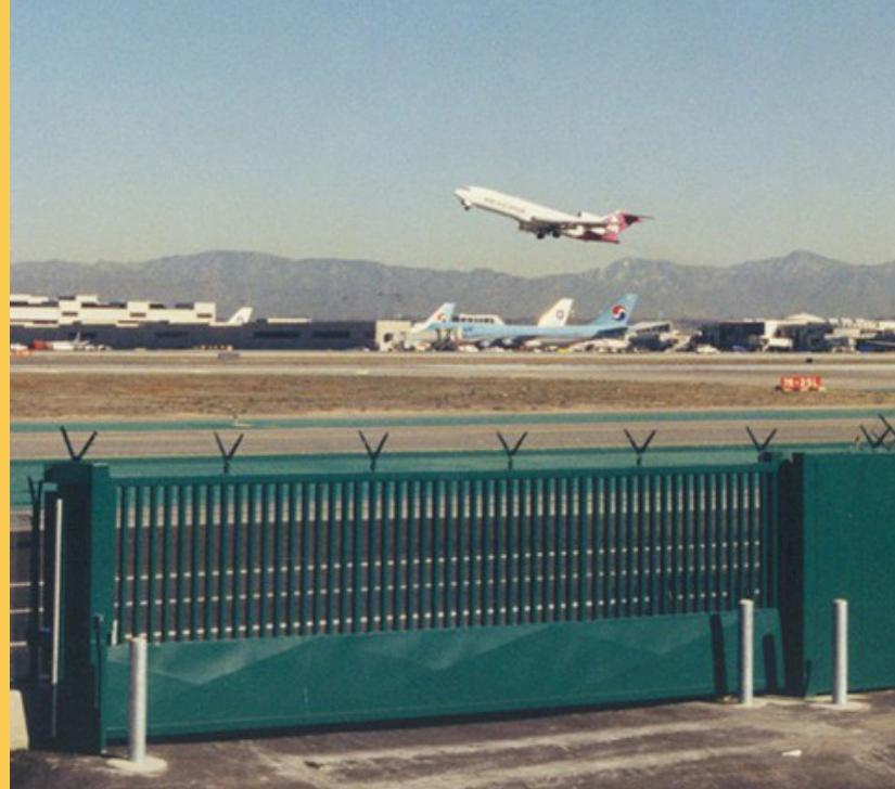
The cantilevered SC3000S sliding gate is ideal for locations that have ground interference and need the leaf of the gate suspended over the roadway. This rugged gate allows for railroad tracks or any other ground obstruction to easily pass underneath the gate leaf during opening and closing of the gate. The drive system can be either electric or hydraulic allowing for variable speeds and smooth operation.
