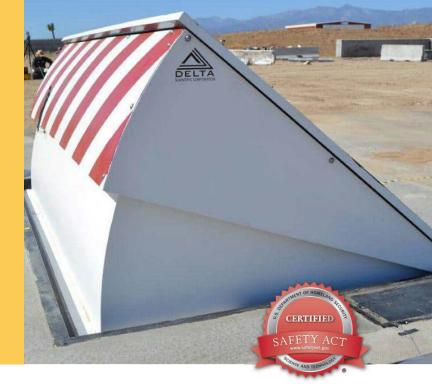
The HD300 barrier, available with either a fully electric or hydraulic control unit, will stop a 15,000 pound (66.7 Km) vehicle traveling 50 mph (80 kpm). Upon impact, the barrier remains in its foundation and the opening stays blocked, providing a multiple hit capability.
