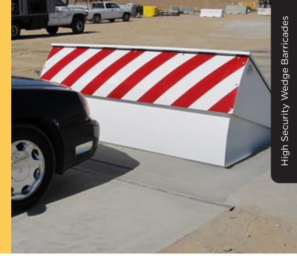
The new Embassy barricade is a fully enclosed, shallow foundation wedge barricade with a covered front and sides. In a full scale crash test conducted by an independent test lab, the DSC207s met the criteria for an M50/ K12 rating. A 15,000 pound (6800 kg) truck impacting at 50 mph (80 km/h) was stopped dead in its tracks with zero penetration and caused no foundation damage. It features a small footprint, a new programmable drive system, and serviceable apparatus.
