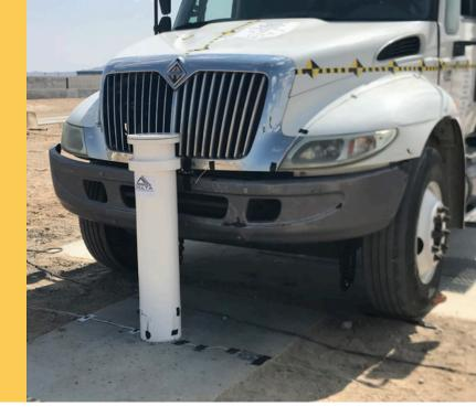
Delta Scientific's new DSC633 shallow foundation bollard single bollard has been successfully tested to ASTM F2656-20 M30/P1 standards. Designed for applications where underground utilities and space limitations pose a problem, the DSC633 is the perfect solution.
