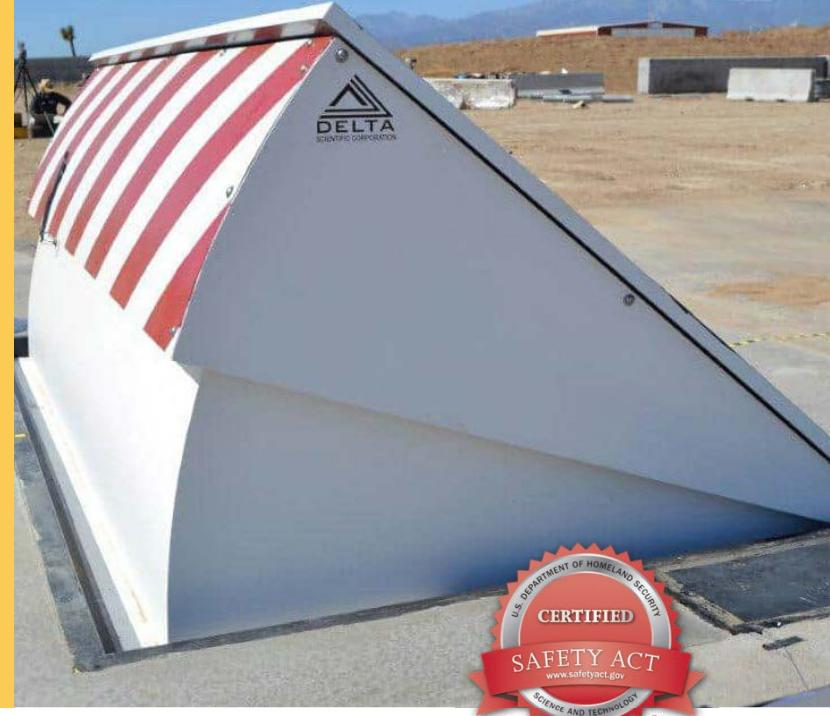
The HD300 barrier, available with either a fully electric or hydraulic control unit, will stop a 15,000 pound (66.7 Km) vehicle traveling 50 mph (80 kpm). Upon impact, the barrier remains in its foundation and the opening stays blocked, providing a multiple hit capability.
