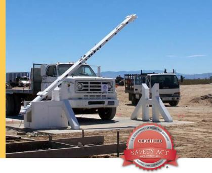
The DSC7000 crash rated beam barricade is used worldwide at locations where wide roadways need to be secured from attacking vehicles. It provides protection between 12- to 20-foot wide with options to 30 feet (3.7 to 9.2 m). The 725-pound beam of the vertical lift barricade stops a 15,000-pound (66.7 kN) vehicle traveling 50 mph (80 kph) dead in its tracks, equivalent to 1.2-million foot-pounds of kinetic energy.
