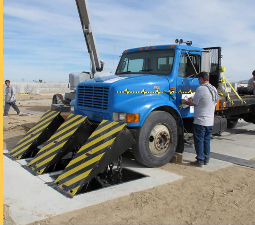
The HD2055 electro-mechanically controlled anti-terrorist barricade decisively stops 15,000 pound (6,803 kg) vehicles traveling at 51 (82 kph) in a recent crash test conducted by an independent testing laboratory. The HD2055 barricades not only stopped the vehicle but contained the test load representing the bombs strapped to the truck bed. The crash test result showed a less than zero penetration.
