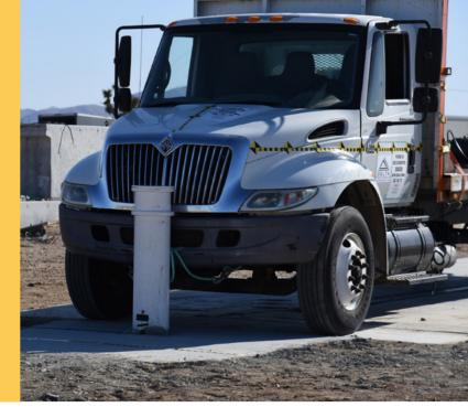
Delta Scientific's new DSC635 shallow foundation single bollard has been successfully tested to ASTM F2656-20 M50/P1 standards. Designed for applications where underground utilities and space limitations pose a problem, the DSC635 is the perfect solution.
