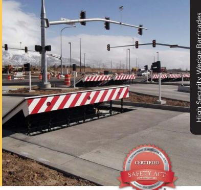
This high security barricade was designed for the U.S. Navy and has also been selected for use at U.S. Embassies. Set in a foundation only 18 inches (46 cm) deep, the Delta DSC501 is able to survive and operate after a 1.2 million foot pound impact. Upon extracting the truck after its crash test, the barricade was fully functional and performed a resounding 27,000 cycles with no wear!
