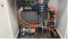
control circuit with an integral motor starter, Power Unit barricade control systems. We rack and stack valves, flow controls and accumulators to meet our client's applications for speed of operation, number of barricades to be controlled and the number of power off cycles required.
