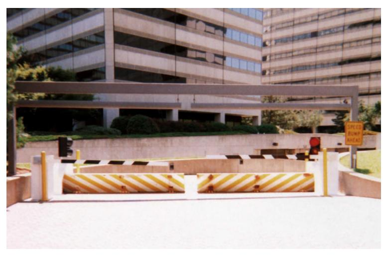
The TW2105 System is designed for controlling normal flow of authorized vehicular traffic yet having the capacity in emergency situations to stop and disable a fast moving vehicle. With all components mounted above grade no cutting or excavation is required on most concrete surfaces provided they meet certain minimum strength and dimensional standards.
