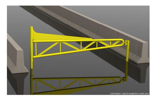
The MG215 is a no nonsense manual swing gate that is available in widths ranging from 12 to 25 feet (3.6 to 7.6 M). It is supplied with the hinge and latching post. It is a robust design that will last for years. The latch consists of a simple cross pin that is pad locked into place. As an option a tamper shield can be provided to protect specific styles of pad locks. Finish is epoxy primer and enamel safety yellow paint.
