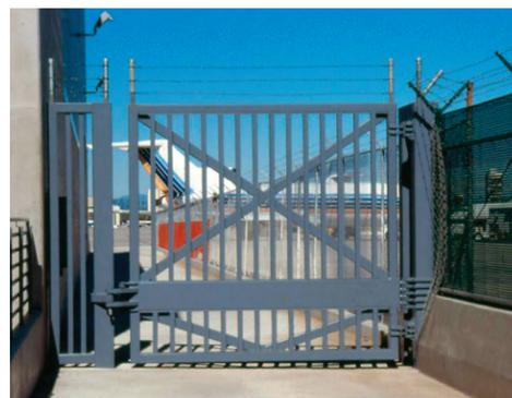
The SGC1000 fills the need for a rugged manual crash-rated swing gate. The design of the end support assemblies add to its crash-rated performance. A ground track is not needed. The SGC1000 provides a clear opening of 12 to 30 feet (3,657 mm to 9,144 mm). The gate can be tailored to match the surrounding decor in a wide variety of architectural treatments.
