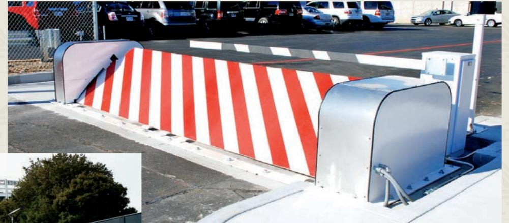
The programmable, electromechanical DSC1450 is a surface mounted vehicle barricade that consists of four components—two buttresses, a road plate and hinge plate. This design provides easy shipment, handling and installation.
