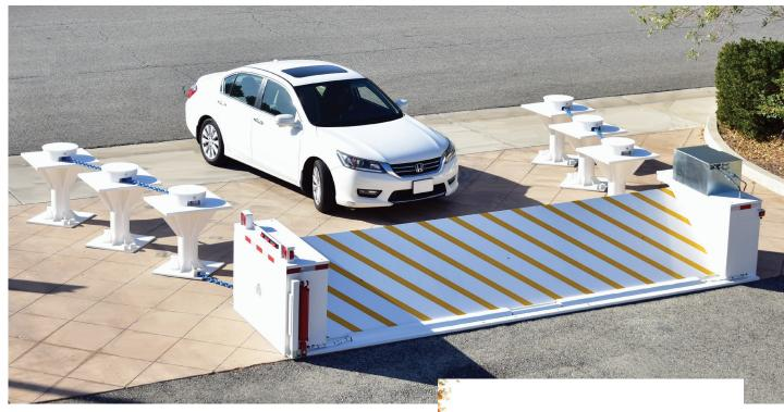
Available now, you can set up certified ASTM M50/P3 rated portable barriers and bollards on concrete, asphalt, compacted soils or vegetation in 15 minutes or less to provide M50 stopping power. Your people are now protected from damage by a 15,000 pound (6804 kg) medium-duty truck going 50 mph (80.4 kph). Quick deployment, multiple configurations and,
