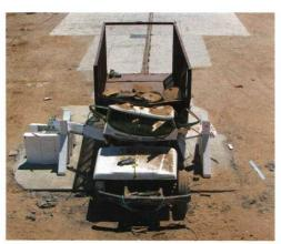
barricade closes in as quickly as 0.7 seconds. The DSC7500 swing beam barricade provides anti-climb features that can replace existing non-rated gates. Both have versions enhanced for nuclear power plants.
