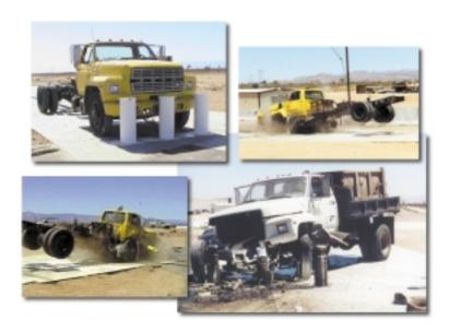
To obtain DOS and DOD certification, Delta bollards were tested to rigorous standards by an independent test laboratory. Full-scale crash tests, using heavily-loaded trucks, were conducted.
