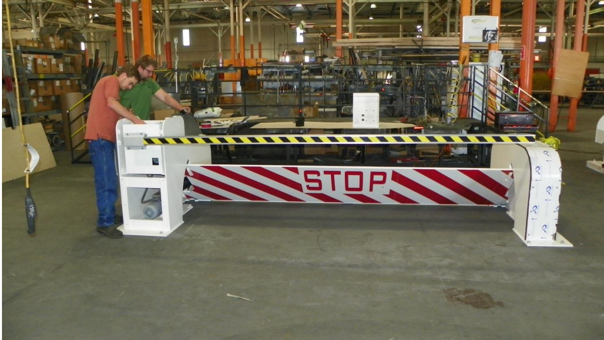
Typical barricade shown in final test. Note stainless steel cover removed.
